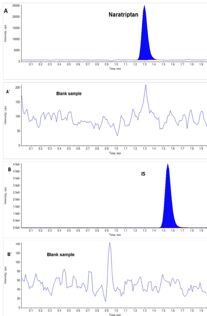
**Figure 2:** Mass chromatograms of blank human plasma spiked with (A) Naratriptan (1.00 ngmL<sup>-1</sup>), (B) Internal Standard (200.00 ngmL<sup>-1</sup>) sample in comparison to the corresponding controls (A' & B') respectively.
