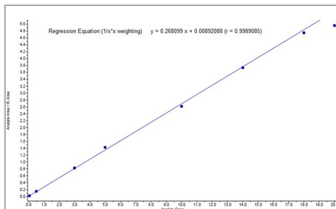
**Figure 4:** Linearity of peak area ratios to the corresponding concentrations of Naratriptan HCl (0.05-20.00 ngmL<sup>-1</sup>)
